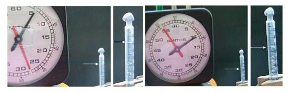
Alternatively, the number of bubbles can be counted and the rate of bubbling calculated. The measuring cylinder was placed above a light source and the bottom masked by varying amounts. The graduations on the flask can provide a convenient guide.
